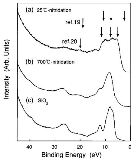
FIG. 3. Synchrotron radiation UPS spectra for the silicon oxide layers nitrided with nitrogen plasma measured at  $h\nu=65$  eV. The nitridation temperature is (a) 25 °C; (b) 700 °C. The spectrum of the silicon oxide layer is included for comparison [spectrum (c)].
