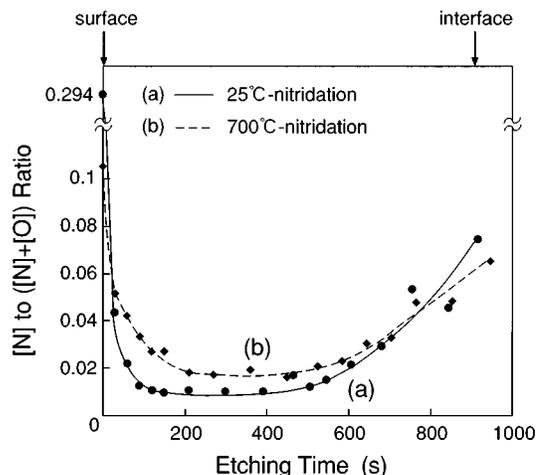
FIG. 2. Depth profiles of the nitrogen concentration ratio,  $\text{N}/(\text{N}+\text{O})$ , for the silicon oxide layers nitrided with nitrogen plasma at the following temperatures: (a)  $25^\circ\text{C}$ ; (b)  $700^\circ\text{C}$ .
