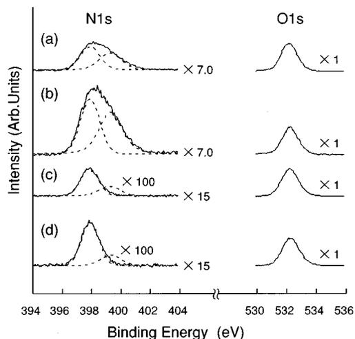
FIG. 1. XPS spectra in the N 1s and O 1s regions for the silicon oxide layers nitrided with nitrogen plasma generated by electron impact. The nitridation temperature,  $T_n$ , and the take-off angle,  $\theta_t$ , are: (a)  $T_n=25^\circ\text{C}$  and  $\theta_t=90^\circ$ ; (b)  $T_n=25^\circ\text{C}$  and  $\theta_t=30^\circ$ ; (c)  $T_n=700^\circ\text{C}$  and  $\theta_t=90^\circ$ ; (d)  $T_n=700^\circ\text{C}$  and  $\theta_t=30^\circ$ .
