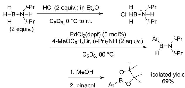
**Scheme 2.** One-pot dehydrogenation/arylation of diisopropylamine–borane with 4-bromoanisole.
