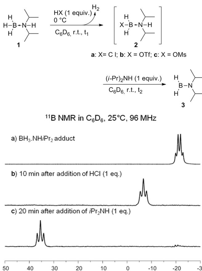
**Figure 1.** Preparation of diisopropylaminoborane:  $^{11}\text{B}$  NMR monitoring ( $\text{C}_6\text{D}_6$ , 25 °C).
