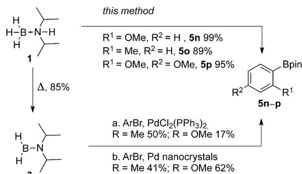
**Scheme 3.** Comparison with reactivity with isolated  $\text{BH}_2\text{N}(i\text{-Pr})_2$  on *ortho*-substituted aryl bromides.
