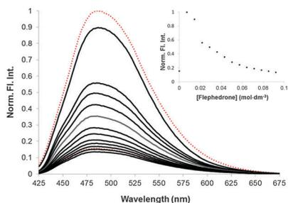
Fig. 4 Normalized fluorescent titration of probe **2** with neat flephedrone (red lines indicate probe **2** only and the first aliquot) Inset: Plot of flephedrone concentration and the quenching of fluorescence intensity at 485 nm (acetone,  $5 \times 10^{-6}$  mol dm $^{-3}$ ,  $\lambda_{\text{ex}} = 410$  nm).
