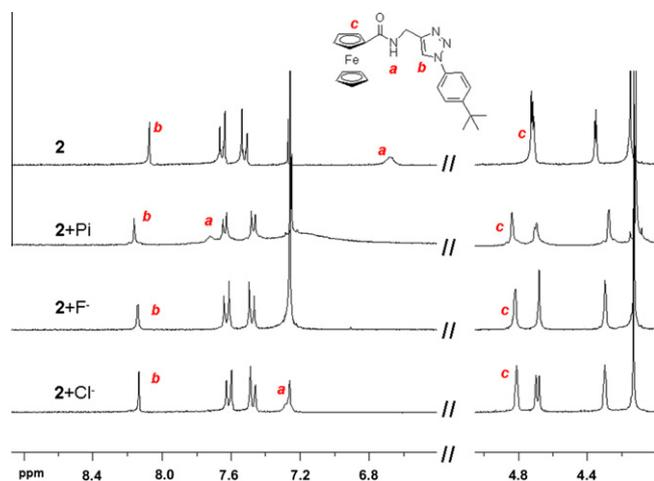
**Figure 4.** Partial  $^1\text{H}$  NMR spectrum of **2** ( $\text{CDCl}_3$ , 27 mM) and after addition 2.0 equiv of  $\text{Cl}^-$ ,  $\text{H}_2\text{PO}_4^-$  and  $\text{F}^-$ .
