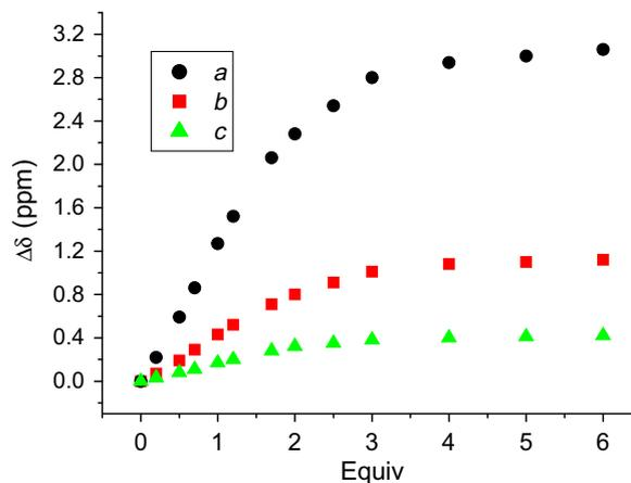
Figure 2. CV titration profile of **1** (0.2 mM) upon addition of various amount of H<sub>2</sub>PO<sub>4</sub><sup>-</sup> in CH<sub>2</sub>Cl<sub>2</sub> solution. Reference electrode = Ag/AgNO<sub>3</sub>; supporting electrolyte = [n-Bu<sub>4</sub>N]PF<sub>6</sub> (0.1 M); scan rate = 100 mV S<sup>-1</sup>.
