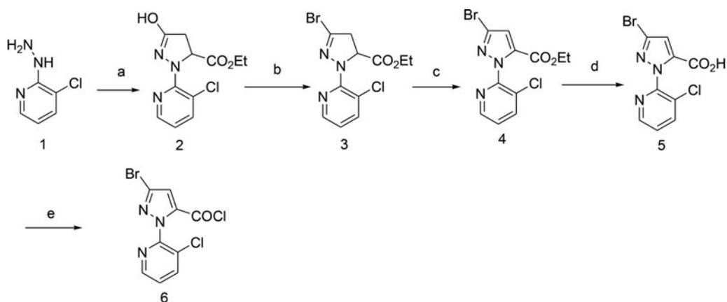
**Scheme 1.** Synthesis of Compounds **6**. Reagents and conditions: (a) diethyl maleate, NaOEt, EtOH, reflux, (b) POBr<sub>3</sub>, MeCN, 80 °C, (c) K<sub>2</sub>S<sub>2</sub>O<sub>8</sub>, H<sub>2</sub>SO<sub>4</sub>, MeCN, reflux, (d) (i) aqueous NaOH, MeOH and (ii) aqueous HCl, (e) SOCl<sub>2</sub>, reflux.
