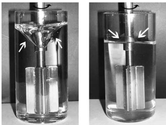
Fig. 2. “Weissenberg effect” 0.01 mol/L Gemini surfactant 15–3–15 aqueous solution (right), compared with distilled water (left) at 800 rpm stirring at the room temperature about 30 °C.
