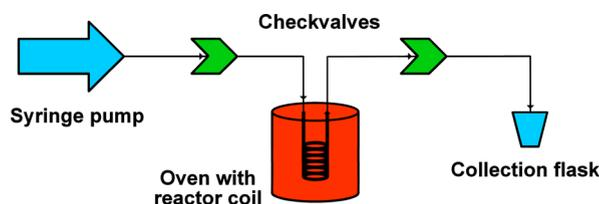
**Figure 1.** Schematic overview of experimental flow setup.
