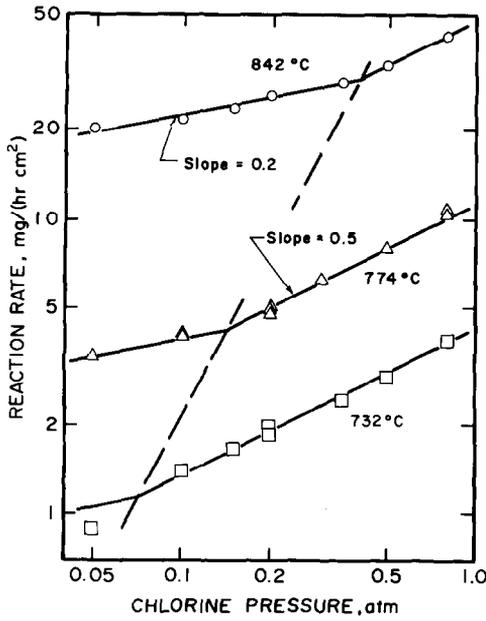
Fig. 3. The effect of chlorine pressure on the chlorination rate of rhenium.
