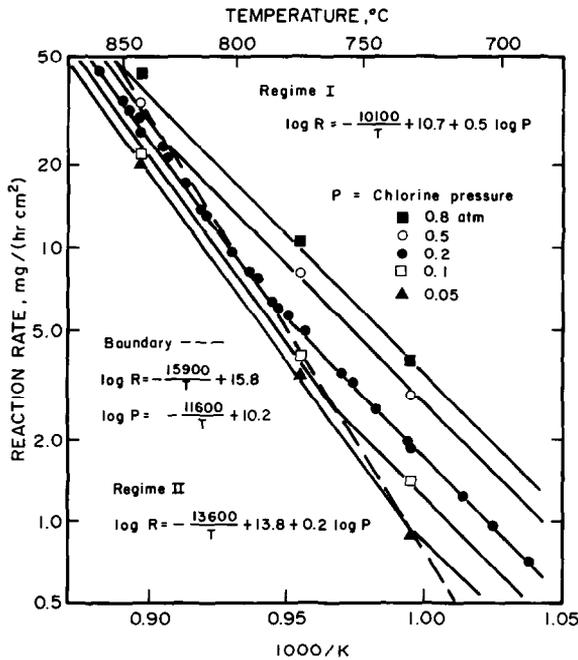
Fig. 4. Complete Arrhenius plot for rhenium chlorination at various chlorine pressures  $P$ : ■,  $P=0.80$  atm; ○,  $P=0.50$  atm; ●,  $P=0.20$  atm; □,  $P=0.10$  atm; ▲,  $P=0.05$  atm; ---, boundary.
