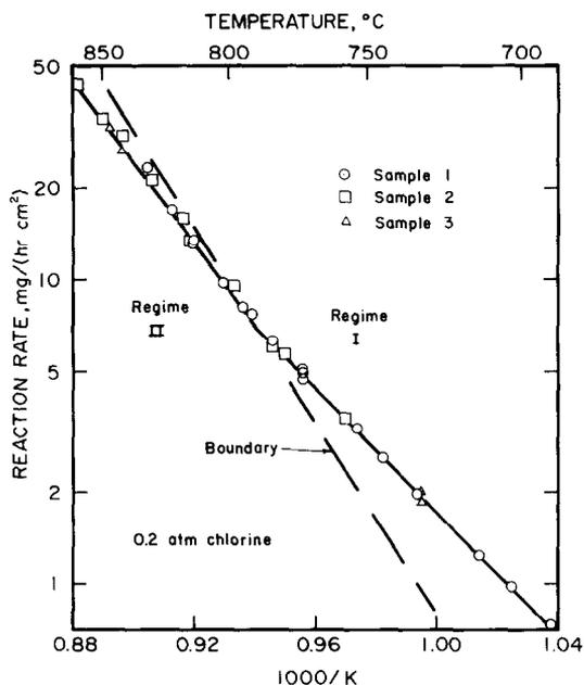
Fig. 2. The Arrhenius plot for the chlorination of rhenium with 0.20 atm of chlorine:  $\circ$ , sample 1;  $\square$ , sample 2;  $\triangle$ , sample 3.
