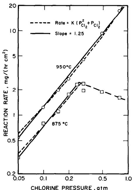
Fig. 7. The effect of chlorine pressures on the chlorination rate of rhodium: ---, rate =  $K(P_{Cl_2}^2 + P_{Cl_2})$ ; —, slope of 1.25.
