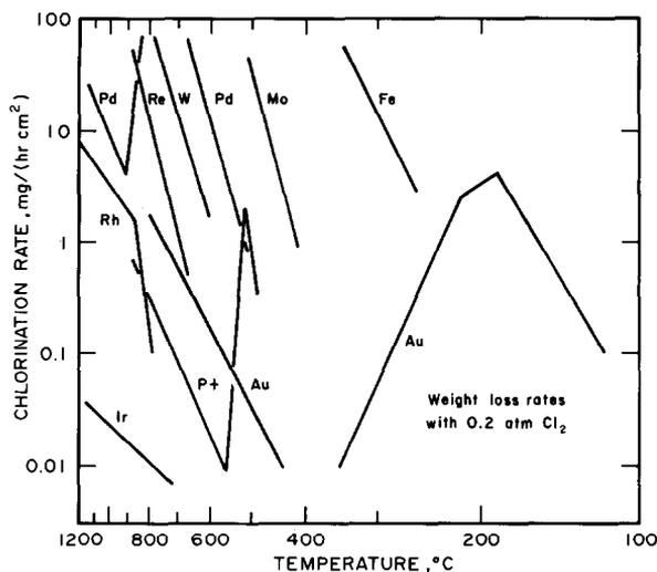
Fig. 1. An Arrhenius plot for the chlorination of several metals (chlorine pressure, 0.20 atm).
