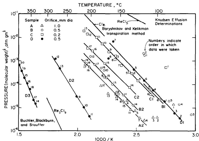
Fig. 5. Chlorine and chloride pressures in the Re-Cl system. The numbers indicate the order in which the data were taken.
