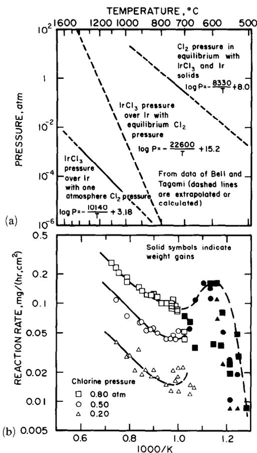
Fig. 8. (a) Vapor and gas pressures (— — —, from data of Bell and Tagami [18, 19]; - - -, extrapolated or calculated) and (b) reaction rates ( $\square$ ,  $P=0.80$  atm;  $\circ$ ,  $P=0.50$  atm;  $\triangle$ ,  $P=0.20$  atm;  $\blacksquare, \bullet, \blacktriangle$ , mass gains) in the Ir-Cl system.
