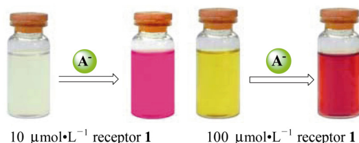
Figure 2 Colour change displayed upon addition of anions ( \text{A}^- = \text{AcO}^- , \text{F}^- and \text{H}_2\text{PO}_4^- ) to receptor 1 at 10 \mu\text{mol} \cdot \text{L}^{-1} and 100 \mu\text{mol} \cdot \text{L}^{-1} .
