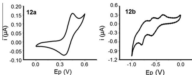
**Figure 2.** Cyclic voltammograms of conjugates 200 μM **12a,b** in HEPES (pH = 7.4) NaClO<sub>4</sub> 1 M, scanning rate: 50 mV s<sup>-1</sup>.
