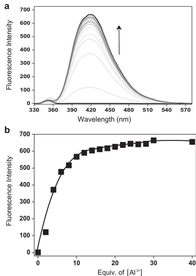
Fig. 3. (a) Fluorescence spectra of CPAP (10  $\mu\text{M}$ ) with different concentrations of  $\text{Al}^{3+}$  in MeOH. (b) Graph of the fluorescence intensity at 420 nm as a function of  $\text{Al}^{3+}$  concentration.
