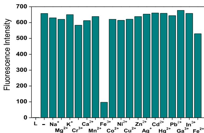
Fig. 4. Relative fluorescence of CPAP alone and its complexation with  $\text{Al}^{3+}$  in the presence of various metal ions. The CPAP response was included as a control (labeled as L). Conditions: 10.0  $\mu\text{M}$  CPAP, 1 equiv metal ions with 1 equiv of  $\text{Al}^{3+}$  ( $E_x = 353$  nm).
