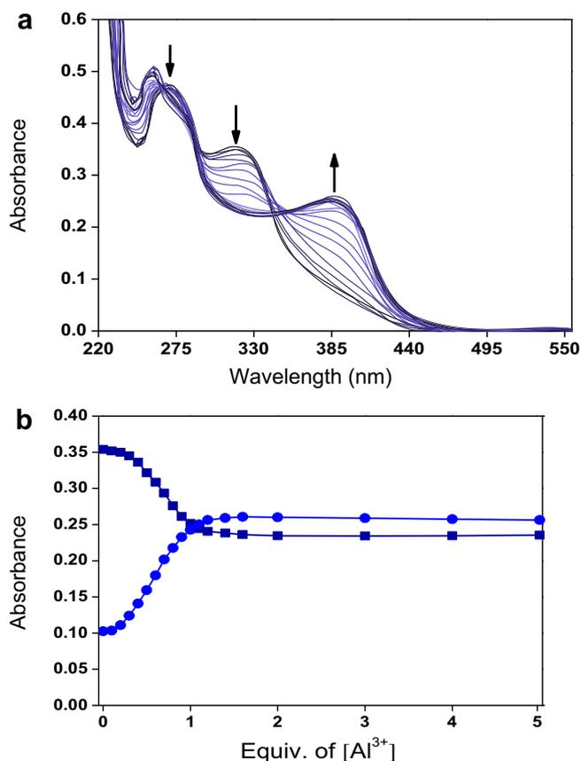
Fig. 1. (a) UV–visible spectral changes in CPAP (40  $\mu\text{M}$ ) after adding aluminum ions (up to 5 equiv) in methanol. (b) Graph of the absorbance at 316 nm (■, squares) and 381 nm (●, circles) as a function of  $\text{Al}^{3+}$  concentration.
