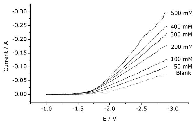
Fig. 3. Slow-sweep voltammograms at a scan rate of  $5$  mV s<sup>-1</sup> of solutions containing various concentrations of nitrate in  $0.1$  M K<sub>2</sub>SO<sub>4</sub>.
