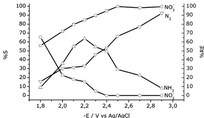
Fig. 10. Influence of the cathodic potential on the distribution of the main products of the reduction of nitrate. The electrolyte was  $0.1$  M  $K_2SO_4/0.05$  M  $KNO_3$  and the electrolysis time was 2.5 h.
