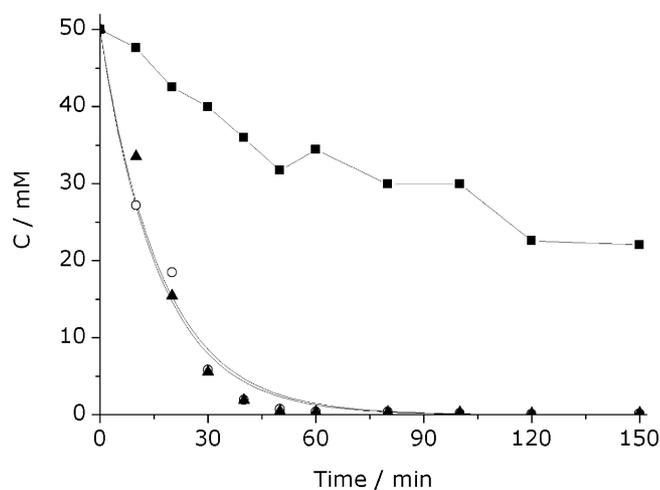
Fig. 7. Concentration profile of nitrate vs. time at: (■) -1.8 V in 0.1 M K<sub>2</sub>SO<sub>4</sub>/0.05 M KNO<sub>3</sub>, (○) at -2.5 V in 0.1 M K<sub>2</sub>SO<sub>4</sub>/0.05 M KNO<sub>3</sub> and (▲) at -2.5 V in 0.1 M K<sub>2</sub>SO<sub>4</sub>/0.05 M KNO<sub>3</sub> + 0.025 M KNO<sub>2</sub>.
