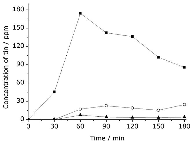
Fig. 6. Concentration of tin in the catholyte vs. time in (■) 0.1 M K<sub>2</sub>SO<sub>4</sub>, (○) 0.1 M K<sub>2</sub>SO<sub>4</sub>/0.05 M KNO<sub>3</sub> and (▲) 0.1 M K<sub>2</sub>SO<sub>4</sub>/0.05 M KNO<sub>3</sub> + 5 × 10<sup>-4</sup> M (NH<sub>4</sub>)<sub>2</sub>SO<sub>4</sub> at -2.9 V vs. Ag/AgCl.
