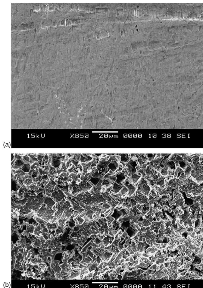
Fig. 5. SEM photograph of (a) an unused and (b) an extensively used for electrolysis tin cathode.
