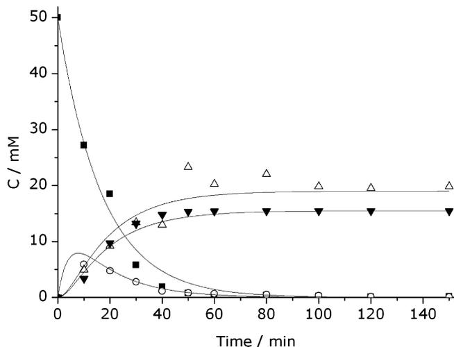
Fig. 8. Variation of the concentration of (■) nitrate, (○) nitrite, (△) ammonia and (▼) nitrogen vs. electrolysis time at  $-2.5$  V. Electrolyte  $0.1$  M  $K_2SO_4/0.05$  M  $KNO_3$ . The lines were drawn by non-linear regression based on the proposed model.
