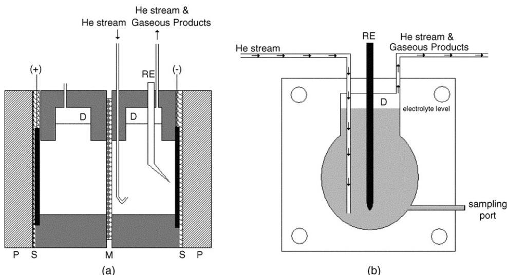
Fig. 1. (a and b) The electrolysis cell: (P) aluminum plates, (S) silicone gasket, (M) nafion membrane, (D) dead volume, (RE) reference electrode. The distance between the Luggin capillary and the cathode was about 1 mm.
