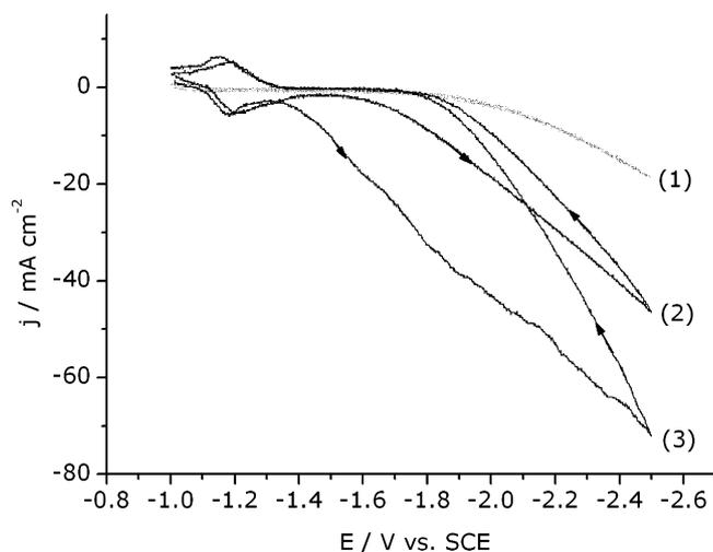
Fig. 2. Cyclic voltammograms in (1) 0.1 M K<sub>2</sub>SO<sub>4</sub>, (2) 0.1 M K<sub>2</sub>SO<sub>4</sub>/0.05 M KNO<sub>3</sub> and (3) 0.1 M K<sub>2</sub>SO<sub>4</sub>/0.05 M KNO<sub>2</sub> electrolyte, at a scan rate of  $50$  mV s<sup>-1</sup>.
