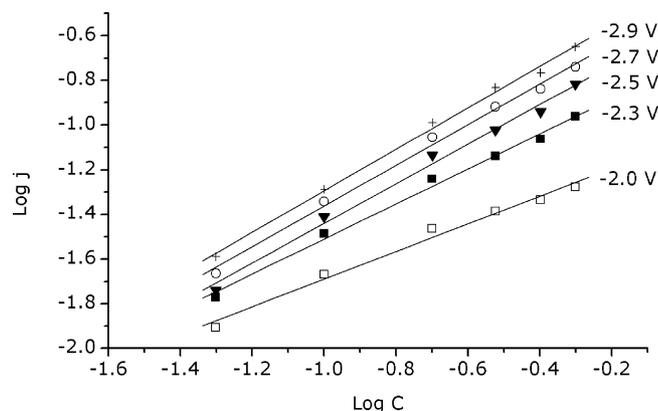
Fig. 4. Logarithm of current density (in A m<sup>-2</sup>) against the logarithm of concentration (in mol L<sup>-1</sup>) at various cathodic potentials.
