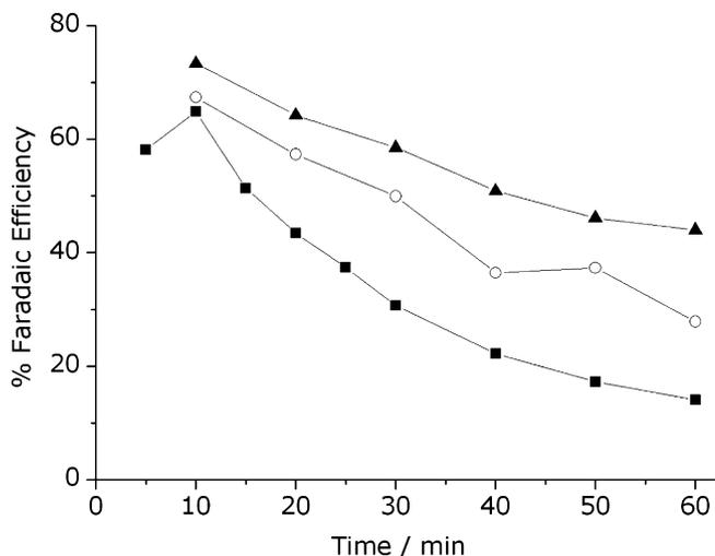
Fig. 9. %Faradaic efficiency of the reduction of nitrate against electrolysis time at (▲)  $-1.8$  V, (○)  $-2.5$  V and (■)  $-2.9$  V. Electrolyte  $0.1$  M  $K_2SO_4/0.05$  M  $KNO_3$ .
