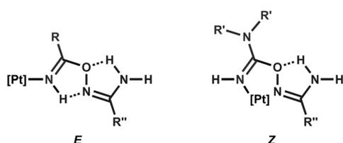
**Figure 1.** *E* configuration (left; for 7, 8, 11–14) and *Z* configuration (right; for 9, 10, 15–17) of the iminoacylated amidoxime ligands.
