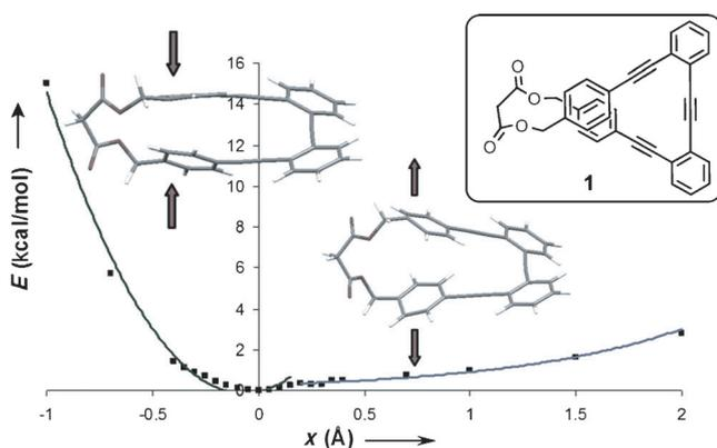
**Figure 3.** Potential energy profile of compound **1** toward elongation.
