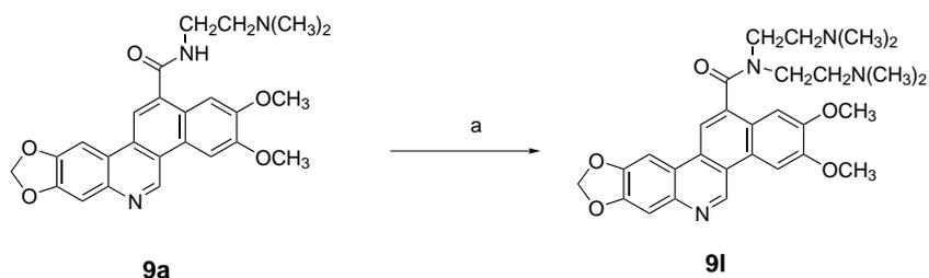
**Scheme 4.** Reagents: (a) NaH, NaI, DMF, ClCH<sub>2</sub>CH<sub>2</sub>N(CH<sub>3</sub>)<sub>2</sub> · HCl.
