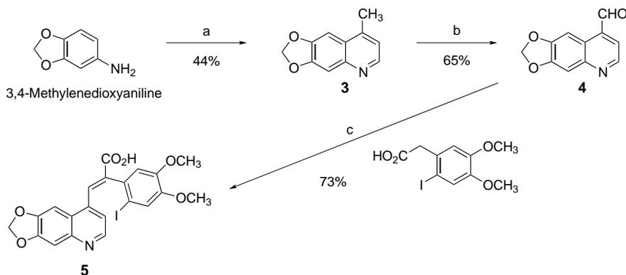
**Scheme 1.** Reagents: (a) Methyl vinyl ketone, FeCl<sub>3</sub>, AcOH (b) SeO<sub>2</sub>, dioxane, H<sub>2</sub>O (c) Ac<sub>2</sub>O, TEA.
