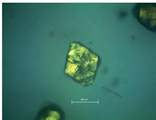
Figure 1. Optical microscopy image of a single crystal of  $\text{K}_2[\text{TcOCl}_5]$ .
