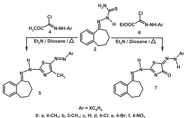
**Scheme 2** Reaction of compounds **2** with hydrazonoyl chlorides **4** and **6**.
