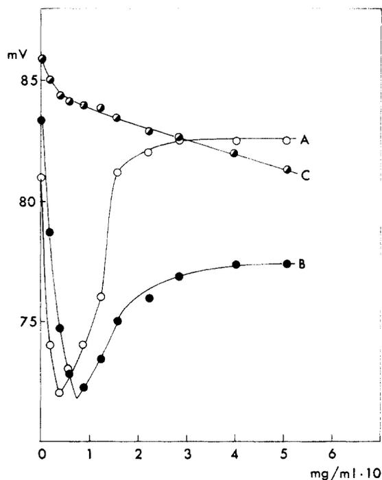
Figure 2.—Electromotive force recorded in a suspension of *E. coli* ( $1 \times 10^{12}$  viable cells/ml) plus  $1 \times 10^{-4}$  M KCl as a function of the increasing concentration of *N*-( $\beta$ -aminoethyl)-polyglycine ( $\overline{DP} = 19$  in plot A;  $\overline{DP} = 6$  in plot B) and of the monomer (plot C).
