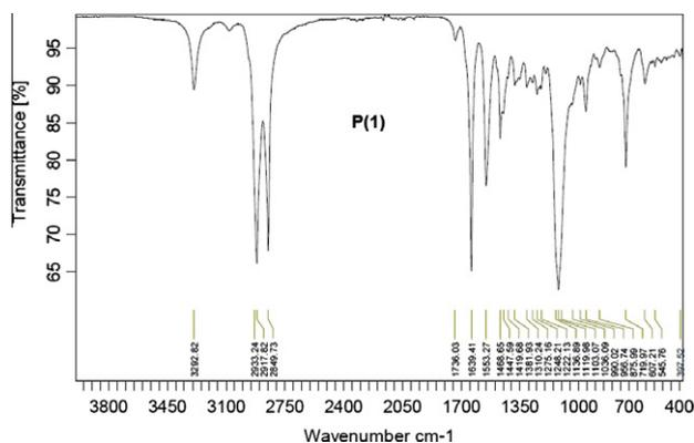
Figure 3. FTIR spectrum of polymer **P(1)**.
