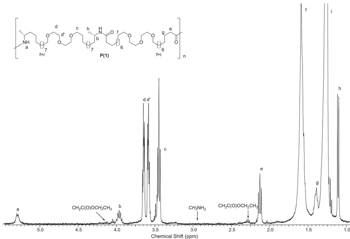
Figure 2.  $^1\text{H}$  NMR spectrum of polymer **P(1)**.
