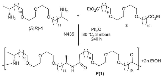
**Scheme 5.** Novozym 435-catalyzed polymerization of monomers (*R,R*)-**1** and **3**.
