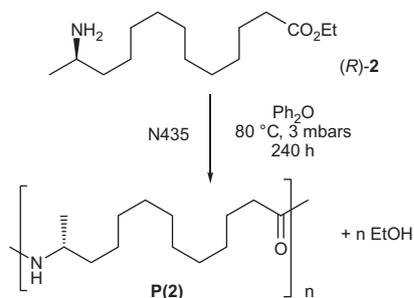
**Scheme 6.** Novozym 435-catalyzed polymerization of monomer (*R*)-**2**.
