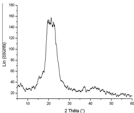
Figure 6. Wide angle X-ray diffraction analysis of polymer P(1).
