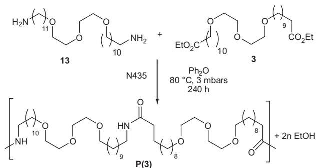
**Scheme 7.** Novozym 435-catalyzed synthesis of model polymer **P(3)**.
