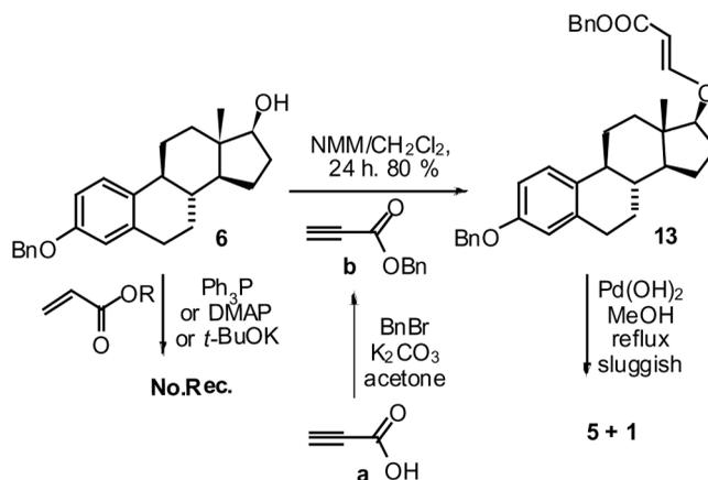
Scheme 4. Synthesis and hydrogenolysis of 13.
