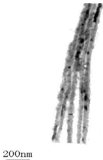
Fig. 2. TEM image of 40 nm diameter and 1.6 \mu\text{m} length Co nanowire arrays.
