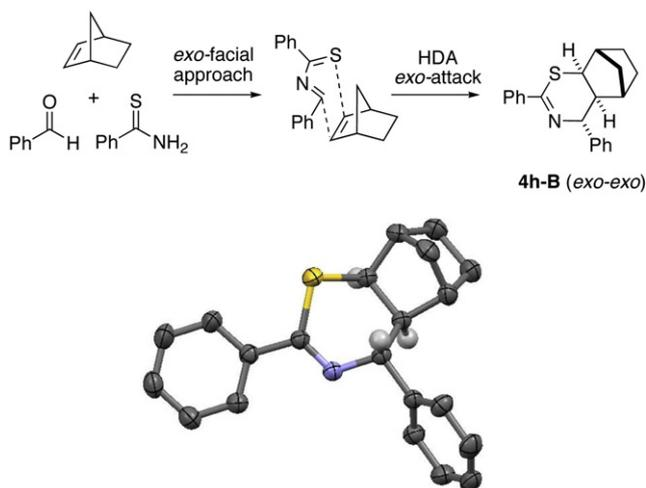
Scheme 3. Reaction of thiobenzamide, benzaldehyde, and norbornene; formation of adduct **4h-B** and its X-ray crystal structure.
