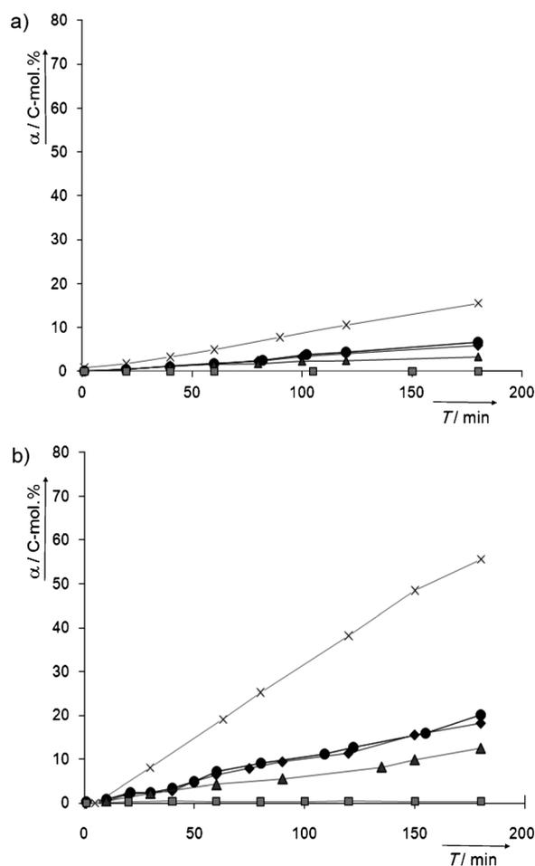
**Figure 4.** GLY conversion: Comparison between a) blank tests and b) GLY oxidation reactions in the presence of gold nanoparticles at NaOH/GLY molar ratios of 4 (x), 3 (●), 2 (◆), 1 (▲), and 0 (■). Reaction conditions: aq. GLY (200 mL, 0.3 M), NaOH/GLY=0–4 (molar ratio), GLY/Au=3500 (catalytic tests, molar ratio), oxygen pressure: 5 bar, temperature: 60 °C.
