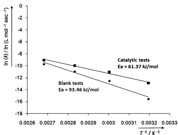
**Figure 10.** Arrhenius plots for gold-catalyzed and base-induced GLY transformations (calculations performed on the basis of initial reaction rates, determined from data in Figure 9).
