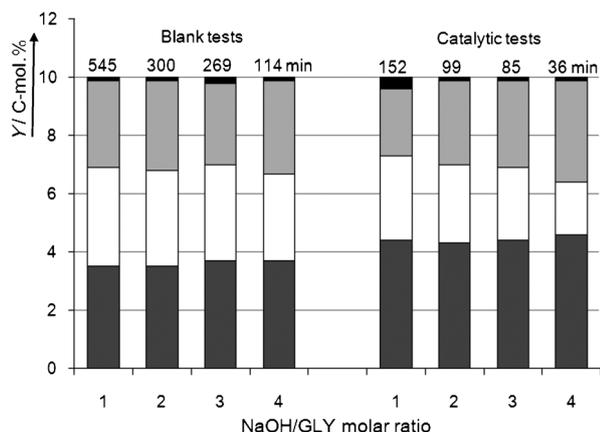
**Figure 5.** Comparison of main product yields [glyceric (■), glycolic (□), and formic acid (▨); tartronic, hydroxypyruvic, and oxalic acid have been summarized (●)] at a GLY conversion equal to 10% for tests with variable base concentrations. Reaction conditions are the same as those reported in Figure 3.
