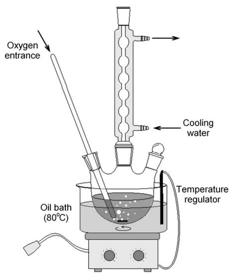
**Figure 11.** Apparatus used for reference test of GLY oxidation in the liquid phase with ultrapure reagents and nonmetallic equipment.
