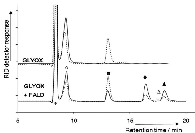
**Figure 15.** Comparison of typical chromatograms of glyoxylic acid (GLYOX, 0.1 M) and its equimolar mixture with formaldehyde (GLYOX + FALD) recorded after 5 (---) and 20 min (—) of reaction in standard conditions (same as those described in Figure 14). The marks represent: sulfuric acid (\*), oxalic acid (○), glycolic acid (◆), glyoxylic acid (■), formaldehyde (△), and formic acid (▲).
