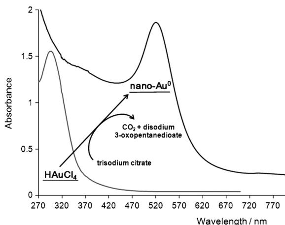
**Figure 1.** Typical UV/Vis spectra of the gold catalyst precursor ( $\text{HAuCl}_4$ ) and gold nanoparticles obtained by the Turkevich method.
