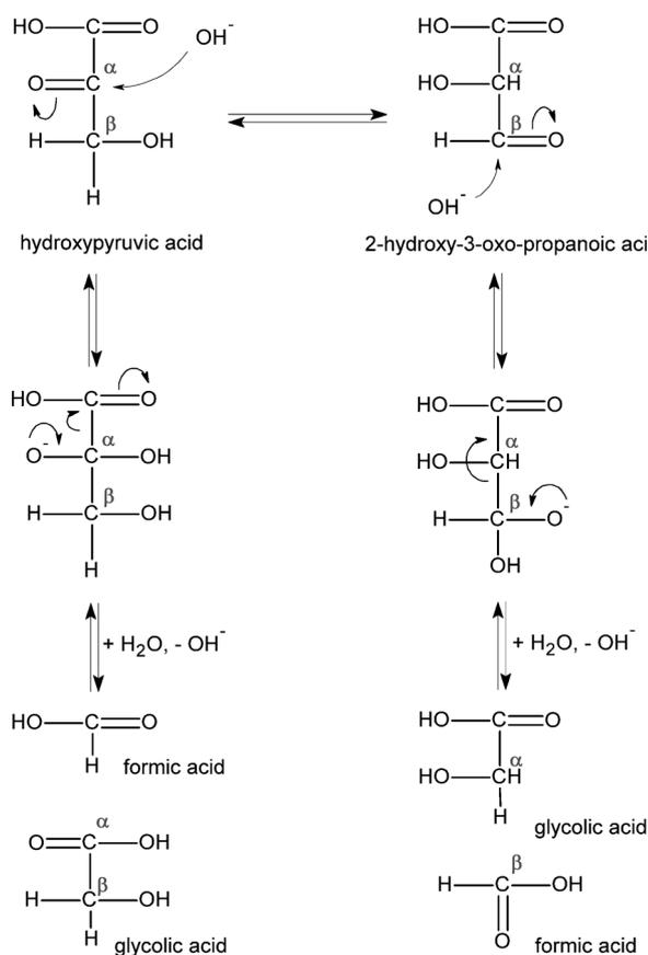
Scheme 6. Possible mechanism of  $\alpha$ - and  $\beta$ -dicarbonyl cleavage.
