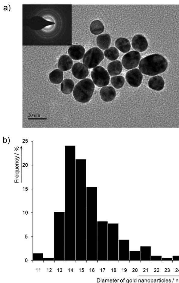
**Figure 2.** a) Representative TEM micrograph and SAED pattern and b) histogram of metal particle size distribution for the solution of gold nanoparticles.
