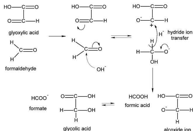
**Scheme 5.** Mechanism of the Cannizzaro cross-reaction for glyoxylic acid and formaldehyde.
