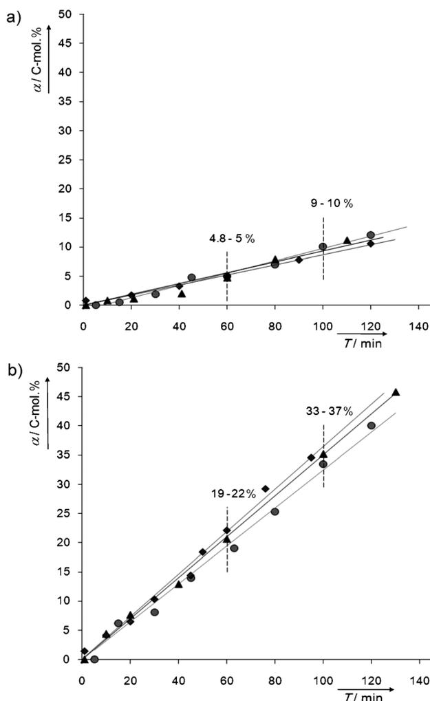
**Figure 8.** Comparison of GLY conversion a) in the absence (blank tests) and b) in the presence of the gold catalyst under variable  $\text{O}_2$  pressure [2.8 (●), 5 (◆), and 10 bar (▲)]. Reaction conditions: aq. GLY (0.3 M), 60 °C, NaOH/GLY = 4 (molar ratio), GLY/Au molar ratio equal to  $\infty$  for blank tests or 3500 for catalytic tests.
