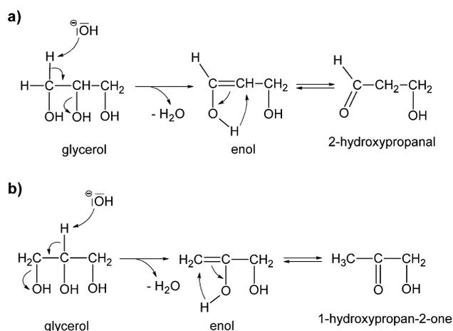
**Scheme 1.** Initial transformation of GLY, which is attacked by the base and, subsequently, the breaking of the a) terminal or b) central C–H bond occurs.
