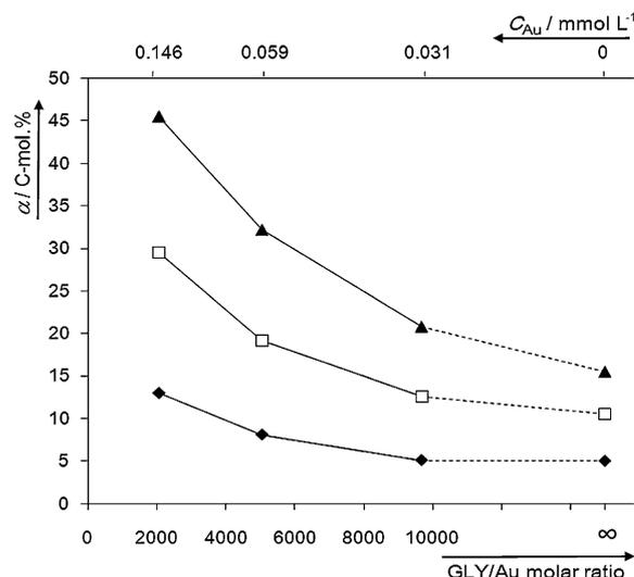
**Figure 6.** Changes in GLY conversion as a function of the GLY/gold molar ratio and reaction time [60 (◆), 120 (□), and 180 min (▲)]. Reaction conditions: aq. GLY (200 mL, 0.3 M), 60 °C, oxygen pressure: 5 bar, NaOH/GLY = 4 (molar ratio).
