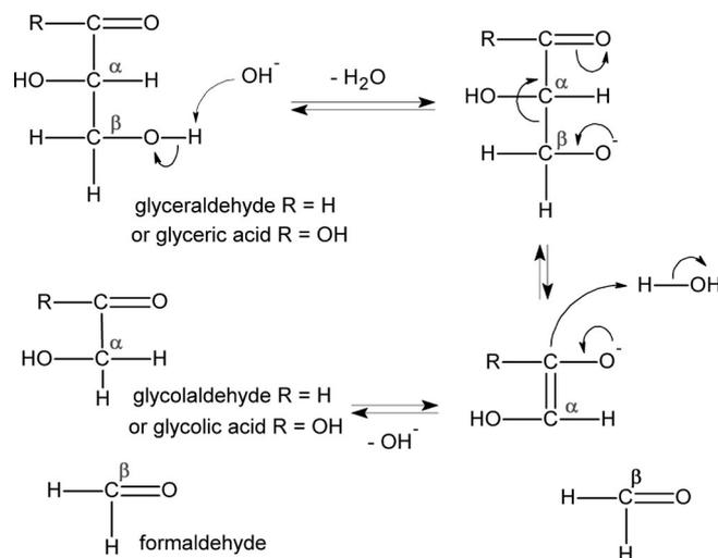
**Scheme 3.** Possible mechanism of the retro-aldol reaction for GLAD and glyceric acid in the presence of a base.
