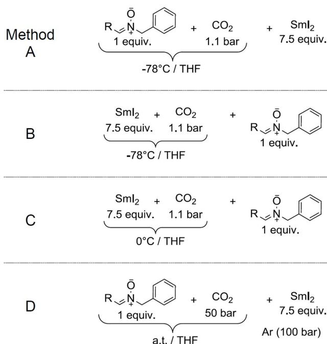
Scheme 3. Reaction conditions and successions of the reagent mixing tested in experiments with nitrones, CO<sub>2</sub>, and SmI<sub>2</sub>.
