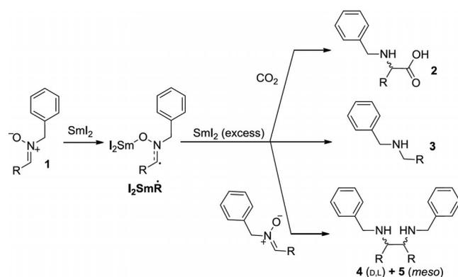
Scheme 2. Possible pathways for the reaction of nitrones with SmI<sub>2</sub> in presence of CO<sub>2</sub>.
