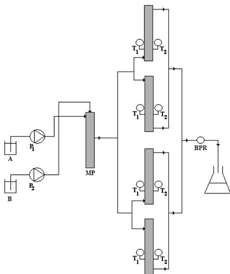
Figure 6. Corning LF reactor with four plates.<sup>31</sup> (A) Nitrile compound in solvent. (B) HA, MP: mixing plate. BPR: back pressure regulator.
