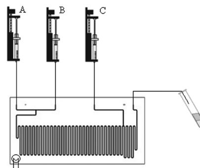
Figure 4. Labtrix S1 microreactor (10  $\mu$ L)<sup>30</sup> A: nitrile compound in solvent, B: HA, C: quenching by solvent.
