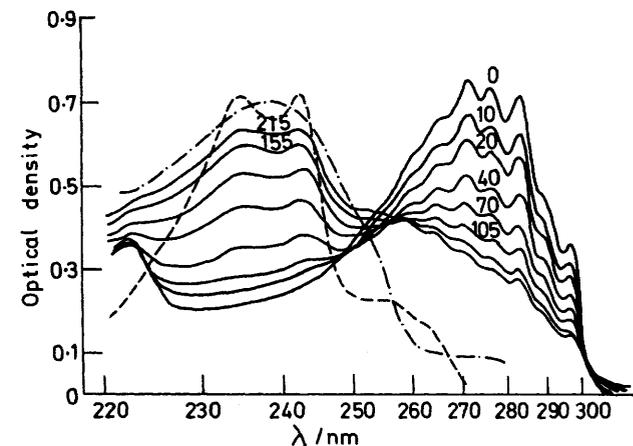
FIGURE 2 Spectral changes (—) of a  $5.03 \times 10^{-5}$  M-solution in cyclohexane of 5-methyl-2-phenyloxazole (23) on irradiation at 294 nm (numbers refer to time in seconds); the spectra of compounds (24) (---) and (25) (- · - · -) in cyclohexane are displayed for comparison
