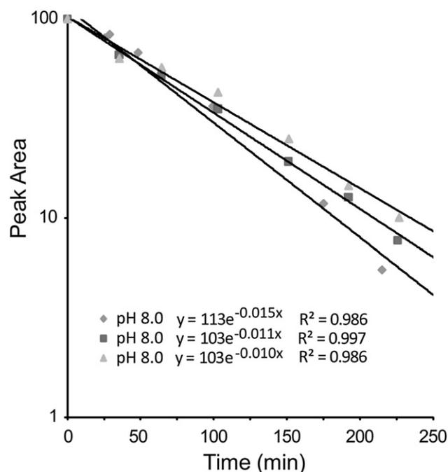
**Fig. 3.** The decline in PB succinimidyl ester  $\mu\text{CE}$  peak area over time at pH 8. Peak areas were normalized to the initial data-collection peak area. Data collected using 100 mM borate, pH 9.5 in separation channel and pH 8 in the sample. Each data point represents one experiment.
