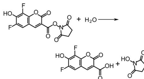
Fig. 1. The hydrolysis reaction of 3-carboxy-6,8-difluoro-7-hydroxycoumarin (Pacific Blue™, PB) succinimidyl ester with water.
