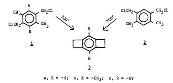
same starting with either 1a or 2, but the pyrolysis of 2 is cleaner and the purification of 3a in this case is easier. Similarly,  $1b^5$  and  $1c^6$  are converted to 3b and 3c, respectively, and in about the same yield. The physical properties of these products are summarized in Table I.
