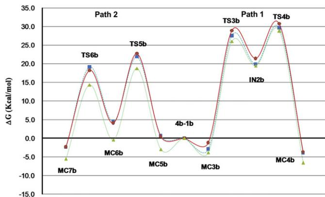
**Fig. 4.** Free energy profile ( $\Delta G$  in kcal/mol), for the reaction of **4b** with **1b**, in vacuo (in blue) in toluene (in red) and in ethanol (in green).
