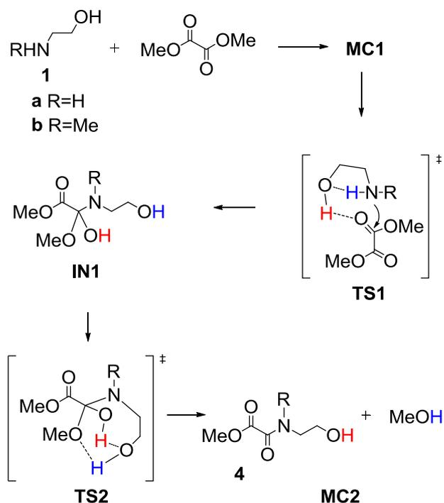
Scheme 2. Mechanism for the conversion of amino alcohols **1a** and **1b** into the intermediate **4**.
