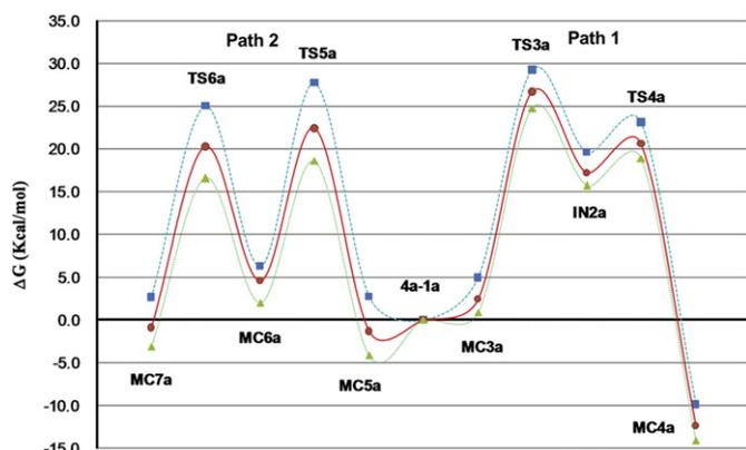
**Fig. 3.** Free energy profile ( $\Delta G$  in kcal/mol), for the reaction of **4a** with **1a**, in vacuo (in blue) in toluene (in red) and in ethanol (in green).
