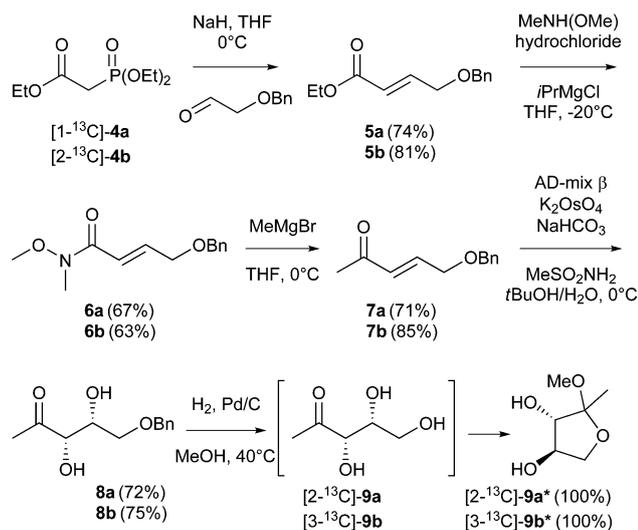
Scheme 1 Synthesis of deoxyxylulose isotopomers **9a** and **9b**.
