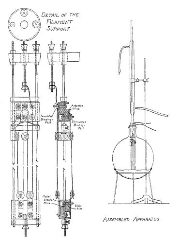
use. Once the filament was in position, it became an easy matter to tighten it, and the resulting tension would cause a depression of the arched spring. Upon passage of the electric current through the filament the expansion which took place was taken up by the tendency of the depressed spring to assume its former position, thus keeping the filament taut at all times. This removed the possibility of short circuiting and eliminated one of the main difficulties of the old apparatus.
