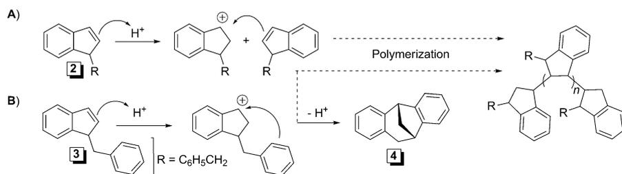
Scheme 1. A) In the presence of acids, indene (**2**, R=H) undergoes a cationic polymerization to give polymeric products. B) In the presence of CH<sub>3</sub>SO<sub>3</sub>H, compound **3** gives dibenzobicyclo[3.2.1]octadiene **4** in 10–77% yield (Table 1).
