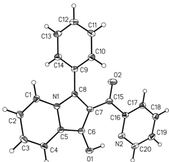
Fig. 1. Molecular structure model and numbering scheme of **3a** as determined by X-ray diffraction investigations (ORTEP, 50% probability ellipsoids, H atoms shown with arbitrary radii).
