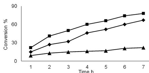
Figure 3. Plot of conversion versus time for styrene carbonate synthesis using catalysts **4**, **6**, and **7**. Triangles, Reaction profiles: ▲ catalyst **4**, ◆ catalyst **6**, ■ catalyst **7**.
