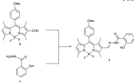
Scheme 1 Synthesis of chemodosimeter 1.
