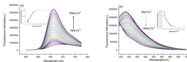
**Fig.2** Fluorescence spectra of chemodosimeter **1** ( $10 \mu\text{M}$ ) towards  $\text{Cu}^{2+}$  (0, 0.02, 0.04, 0.08, 0.1, 0.3, 0.5, 0.8, 1, 2, 3, 4, 5, 6, 7, 8, 9, 10, 11, 12, 13, 14, 15, 18, 23, 30, 40 equiv) in DMF: $\text{H}_2\text{O}$  (7:3, v:v) medium, (a)  $\lambda_{\text{ex}} = 450 \text{ nm}$ , (b)  $\lambda_{\text{ex}} = 525 \text{ nm}$ .
