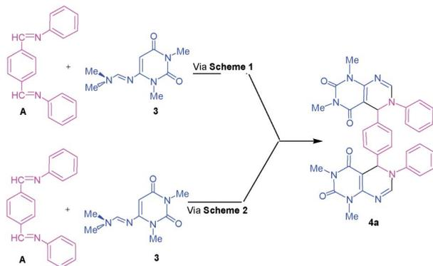
Scheme 3 Synthesis of bis-pyrimido[4,5-*d*]pyrimidine derivative (**4a**).
