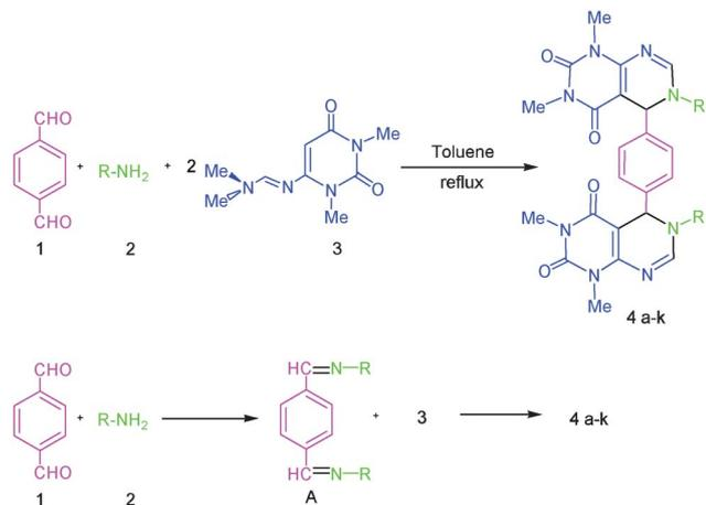
Scheme 1 Synthesis of bis-pyrimido[4,5-*d*]pyrimidine derivatives (4a–k).
