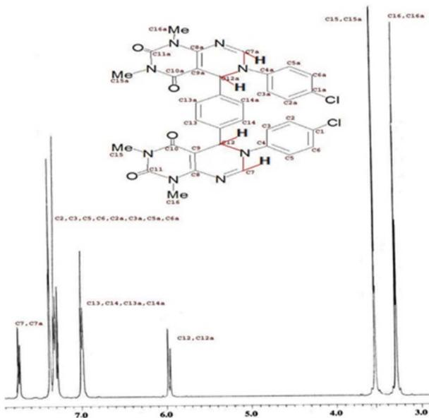
Fig. 1 The  $^1\text{H}$  NMR spectrum of **4b**, which shows the long range *W*-coupling constant.
