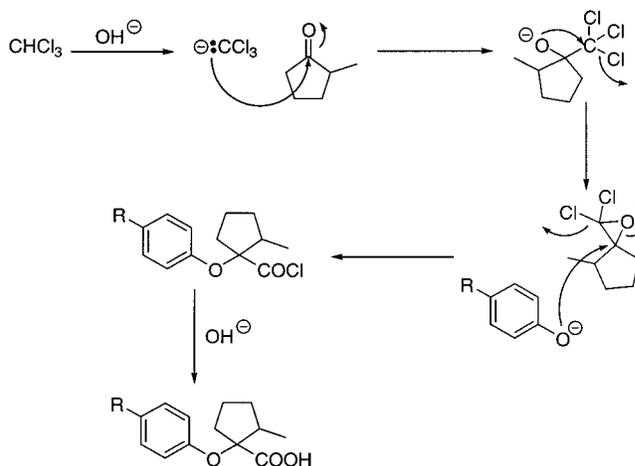
**Figure 3.** Mechanism for the ketone–chloroform reaction in the synthesis of compound **11**.
