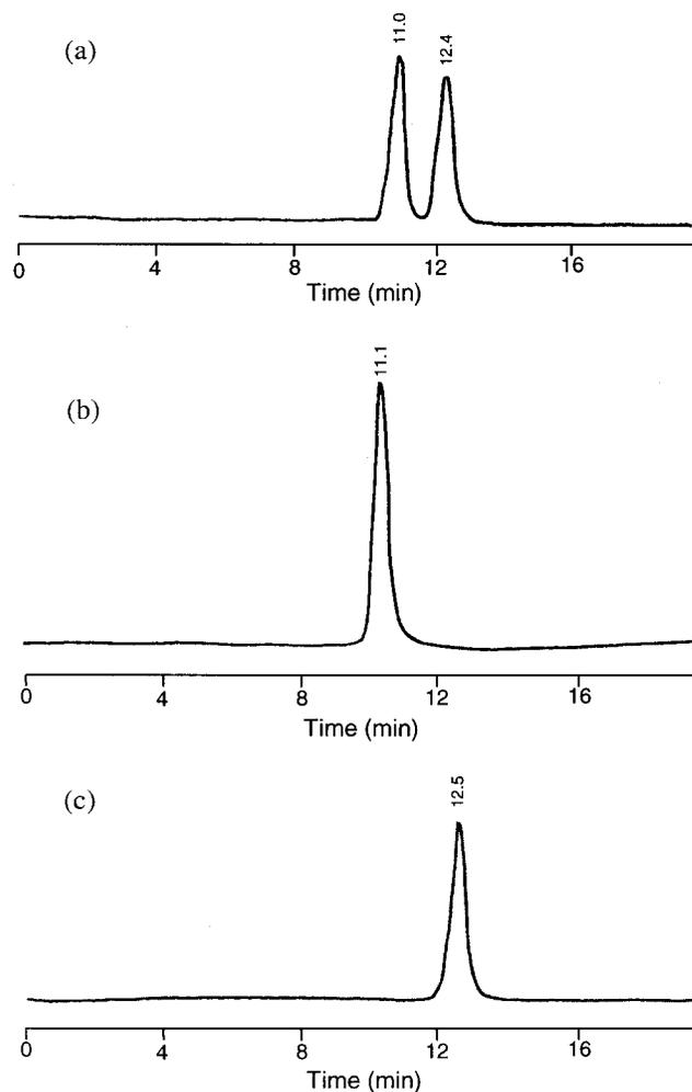
**Figure 2.** HPLC enantioseparation of (a) racemic mixture (±)-**10**, (b) (–)-**10**, and (c) (+)-**10**. Conditions: Chiracel OD (0.46 × 25 cm); mobile phase 90:10 heptane/ethanol with 1% TFA; flow rate 1.0 mL/min; detection wavelength 254 nm.
