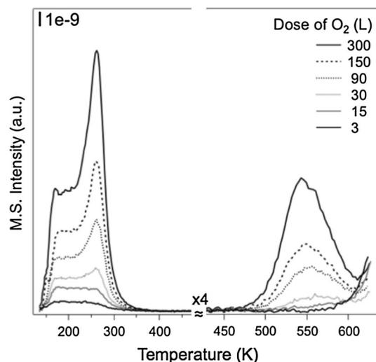
**Fig. 1** Evolution of adsorbed molecular and atomic states of oxygen following dosing of the npAu surface with oxygen in UHV. Dioxygen dosed from 3 to 300 Langmuir at 130 K shows molecular desorption at 170 and 270 K and atomic recombination near 550 K. A nearly linear heating rate of 3 K s<sup>-1</sup> was used. The sample was prepared by cleaning at 300 K in UHV with a direct dose of an ozone-rich oxygen followed by 130 annealing cycles up to 600 K observing methanol oxidation
