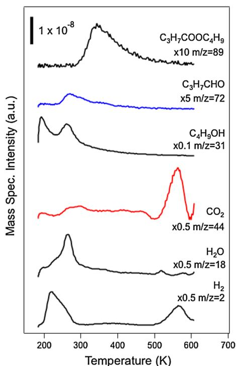
**Fig. 3** Temperature programmed reaction of 1-butanol on npAu. 30 Langmuir of dioxygen was dosed at 300 K to achieve 10 % saturation coverage. Subsequently, 1.0 Langmuir of 1-butanol was dosed at 180 K. Overlapping mass fragments have been subtracted for clarity. The heating rate was approximately  $3 \text{ K s}^{-1}$
