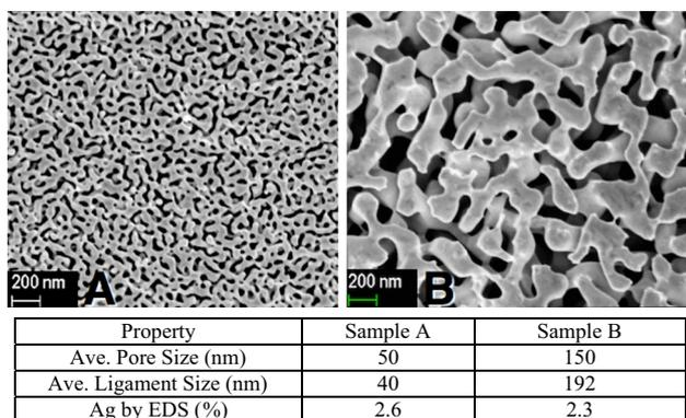
**Fig. 5** Scanning electron micrograph (SEM) images of the npAu catalyst before reactions in ultrahigh vacuum (a) and after (b) ozone treatment and reactions. The ligament structure has increased from ~50 nm in pore and ligament size to ~160 nm while retaining activity for oxidative coupling
