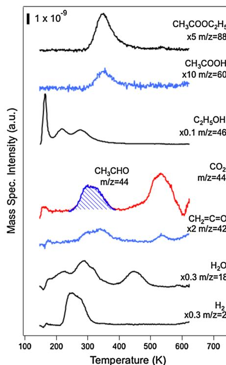
**Fig. 2** Temperature programmed reaction of ethanol on npAu. 60 Langmuir of dioxygen was dosed at 300 K to achieve 10 % saturation coverage. Subsequently, 1.5 L ethanol was dosed at 140 K. Overlapping mass fragments have been subtracted for clarity. The  $m/z = 44$  mass indicates acetaldehyde evolution at 300 K (shaded) and  $CO_2$  evolution at 550 K. The heating rate was  $3\text{ K s}^{-1}$
