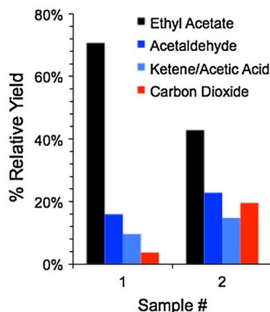
**Fig. 6** Product distributions of a nanoporous gold catalyst before (1) and after (2) 65 different reactions with annealing to 600 K. Initial oxygen coverages were approximately 20 % of surface oxygen saturation
