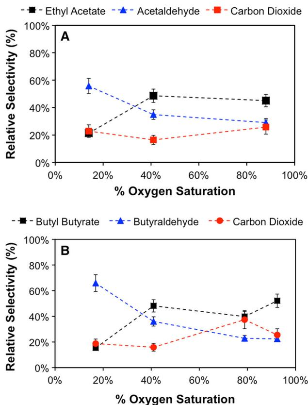
**Fig. 4 a** Selectivity dependence on oxygen coverage for ethanol oxidation. Dioxygen was dosed at 300 K from 15 to 300 Langmuir to obtain 20–95 % saturation coverage. **b** Selectivity dependence on  $\text{O}_2$  for 1-butanol oxidation. Dioxygen was dosed at 300 K from 1.5 to 15 Langmuir. Conversion and selectivity were obtained from TPRS data at each  $\text{O}_2$  coverage. Lines are drawn to direct the eye only
