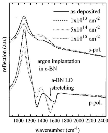
FIG. 2. PIRR data (wire grid polarizer on  $\text{CaF}_2$  substrate,  $\Phi=60^\circ$ ,  $\alpha=90^\circ$ ) before and after implantation with argon (40 keV) at different doses.
