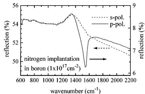
FIG. 4. PIRR data ( $\Phi=60^\circ$ ) of a boron film with a nitrided surface layer using plasma immersion ion implantation.
