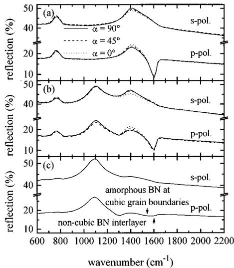
FIG. 1. PIRR data ( $\Phi=45^\circ$ ) taken at different angles  $\alpha$  for (a) a noncubic BN film ( $I/A=1.6$ ), (b) a  $c$ -BN containing film ( $I/A=1.8$ ), and (c) a highly cubic film ( $I/A=2.0$ ). The plane of incidence of the IR beam was rotated in (a) and (b).
