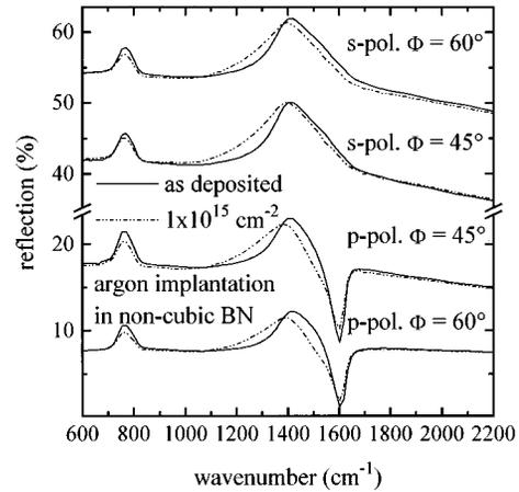
FIG. 3. PIRR data ( $\alpha=90^\circ$ ) of non-cubic BN before and after argon (40 keV) implantation.
