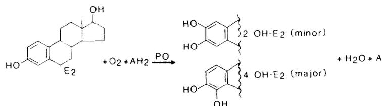
Fig. 2. Reaction scheme for the bioconversion of  $E_2$  into 2OH- $E_2$  and 4OH- $E_2$  by *Mucuna*-phenoloxidase (PO). Na-ascorbate ( $AH_2$ ) serves as a co-factor and an anti-oxidant, to prevent quinone formation.
