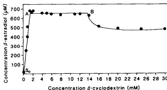
Fig. 1. Phase-solubility diagram of the  $E_2/\beta$ -CD system at  $25^\circ$ .
