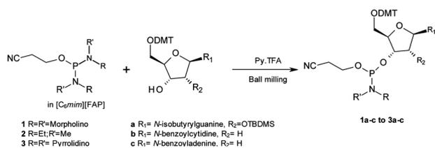
**Fig. 1** Schematic representation of the reaction of phosphorodiamidites to form nucleoside phosphoramidites using mechanochemistry and a stabilising IL.
