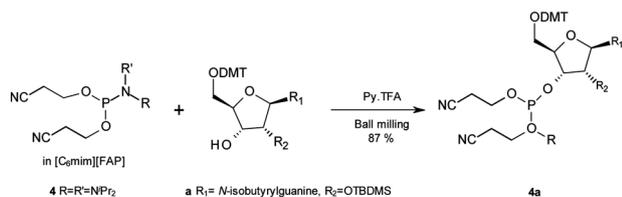
**Fig. 2** Synthesis of **4a** from partially protected guanosine and phosphoramidite **4** using ball milling conditions.
