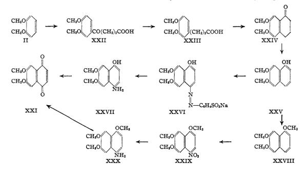
the known 1,6,7-trimethoxynaphthalene (XXVIII) followed by nitration to 4-nitro-1,6,7-trimethoxynaphthalene (XXIX). The nitro compound was then catalytically reduced and the resulting amine (XXX) oxidized to the quinone (XXI).
