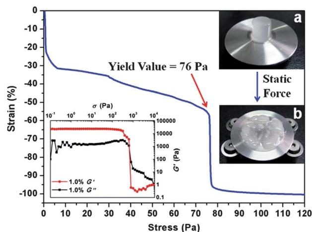
**Fig. 1** Static compression strain vs. stress curve of a cylinder ionogel of **1D**/IL2 at 10 mg mL<sup>-1</sup> and its rheological behaviors (left inset), the cylinder ionogel before (a) and after (b) compression (right inset).
