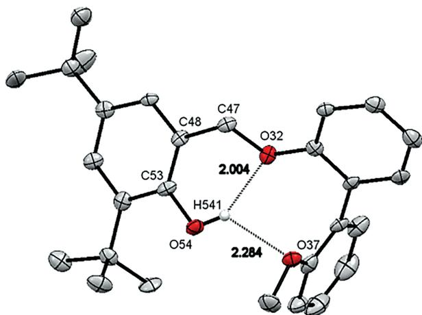
Figure 3. ORTEP diagram of the molecular structure of ligand **3a** (CCDC-1405437). The thermal ellipsoids are shown at the 50% probability level. Hydrogen atoms are omitted for clarity except for the phenolic hydrogen atom. Selected bond length [Å] and angles [°]: C53–O54 1.392(6), C47–O32 1.467(6), O54–H541 0.855(3), O32–H541 2.004(3), O37–H541 2.284(4); C48–C53–O54 122.0(4), C48–C47–O32 107.9(4), C53–O54–H541 103.8(3).
