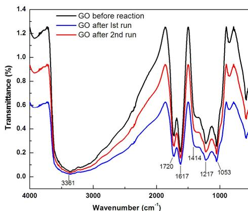
Fig. 4 Comparative FT-IR spectra of GO before use (black), after 1<sup>st</sup> (blue) and 2<sup>nd</sup> run (red).
