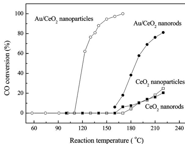
**Figure 7.** Catalytic activities of CeO<sub>2</sub> nanorods and Au/CeO<sub>2</sub> nanorods (solid) as compared with CeO<sub>2</sub> nanoparticles and Au/CeO<sub>2</sub> nanoparticles (open) at different reaction temperatures.
