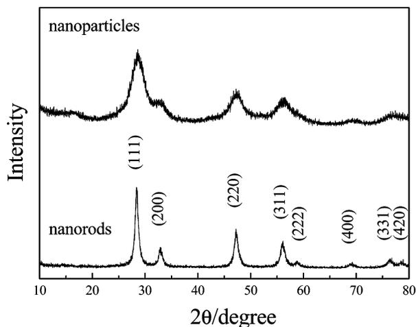
**Figure 2.** XRD patterns of the CeO<sub>2</sub> nanorods synthesized at 180 °C for 45 h and CeO<sub>2</sub>·*n*H<sub>2</sub>O nanoparticles.
