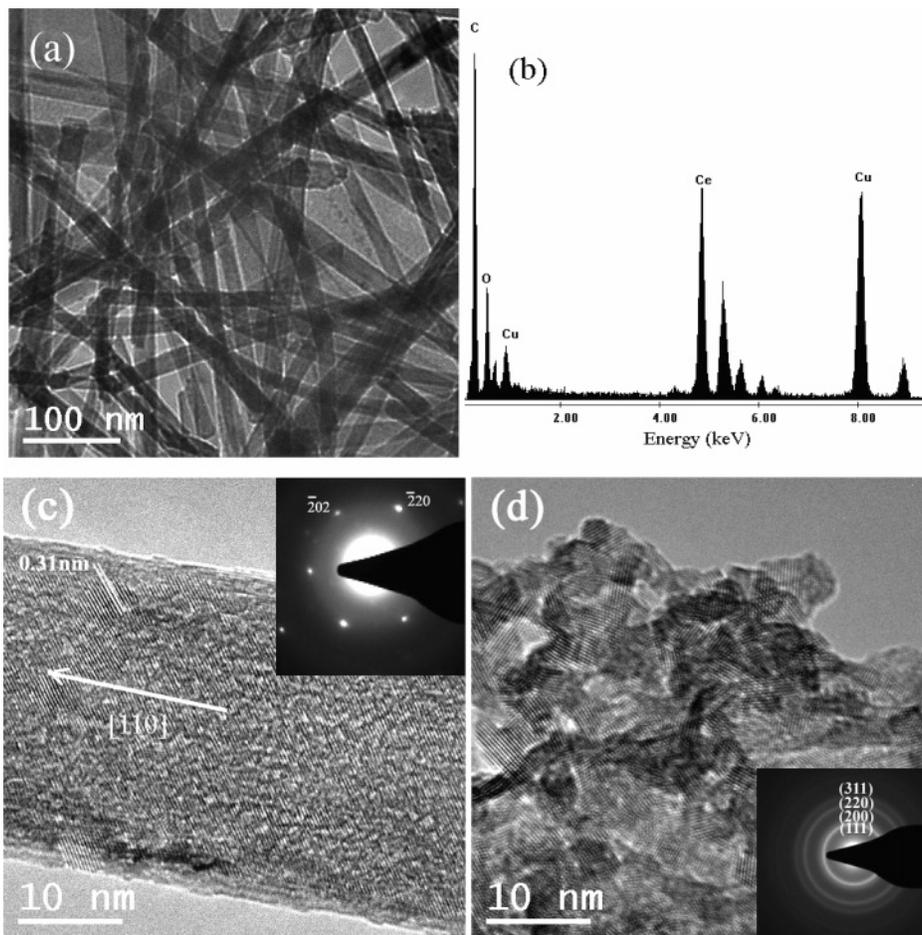
**Figure 4.** TEM images (a) and EDS (b) of the  $\text{CeO}_2$  nanorods synthesized at  $180^\circ\text{C}$  for 45 h. The HRTEM images of the  $\text{CeO}_2$  nanorods and  $\text{CeO}_2 \cdot n\text{H}_2\text{O}$  nanoparticles are shown in c and d. The inserts in c and d are SAED of individual  $\text{CeO}_2$  nanorod and  $\text{CeO}_2 \cdot n\text{H}_2\text{O}$  nanoparticles, respectively.
