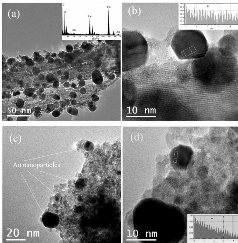
**Figure 5.** TEM and HRTEM images of Au/CeO<sub>2</sub> nanorods (a and b) and Au/CeO<sub>2</sub> nanoparticles (c and d). The EDS spectrum of Au/CeO<sub>2</sub> nanorods is inserted in a.
