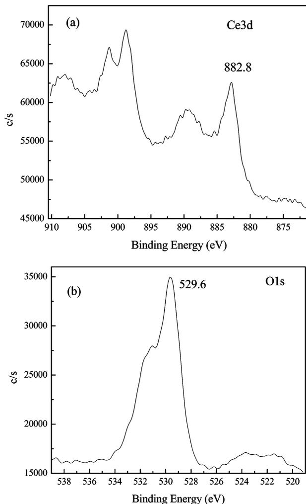
**Figure 3.** Ce3d (a) and O1s (b) core level spectra observed for CeO<sub>2</sub> nanorods synthesized at 180 °C for 45 h.
