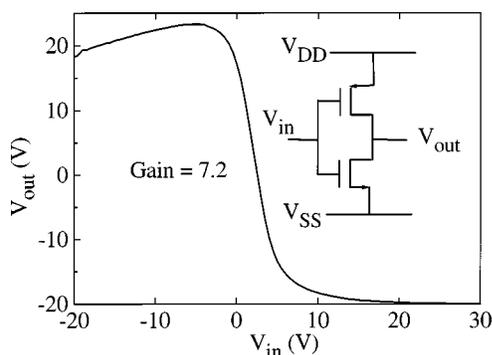
FIG. 3. Voltage transfer characteristics of a CMOS inverter made of  $\mu c$ -Si. The  $p$  channel and  $n$  channel TFTs have identical channel dimensions.  $V_{DD}=30$  V and  $V_{SS}=-20$  V.
