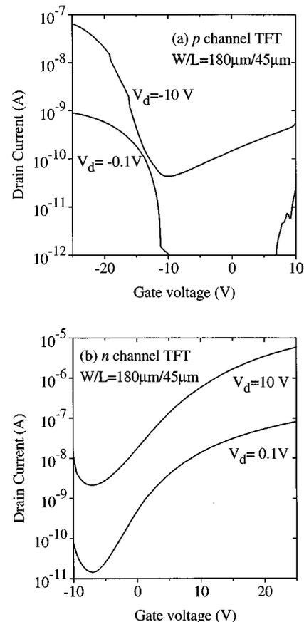
FIG. 2. Transfer characteristics of the (a)  $p$  channel  $\mu c$ -Si TFT, and (b)  $n$  channel  $\mu c$ -Si TFT of the CMOS inverter.
