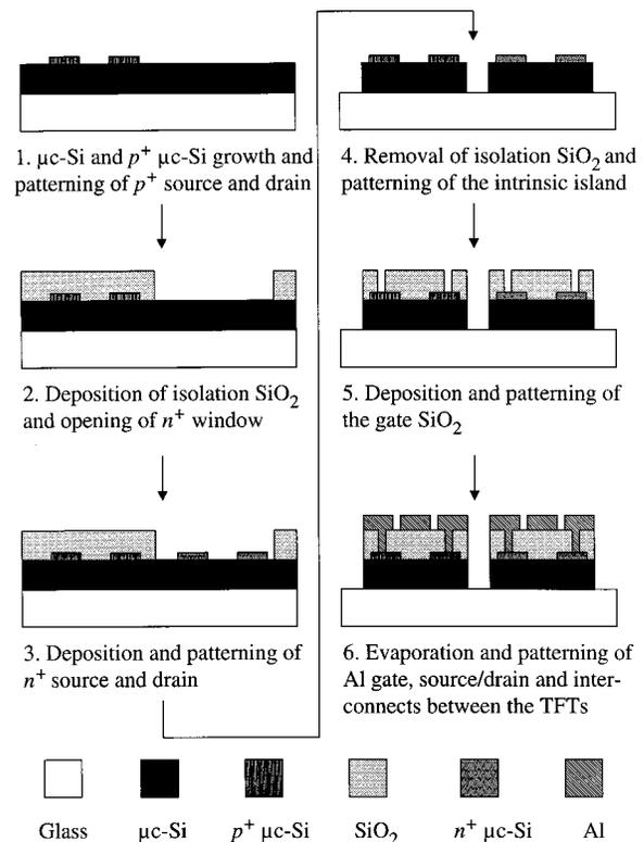
FIG. 1. Schematic process sequence for the microcrystalline silicon CMOS inverter.
