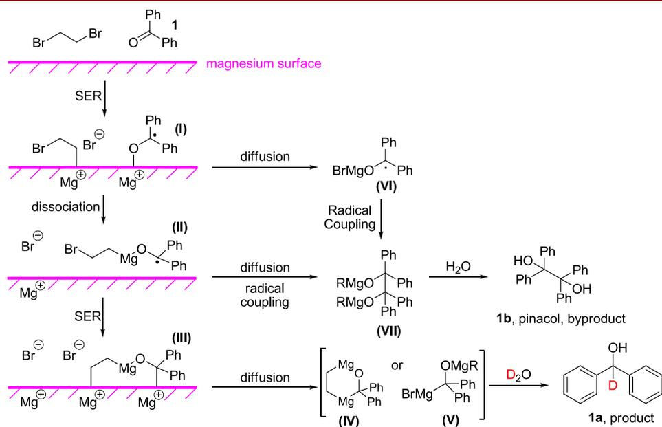
Figure 5. Proposed mechanism for the reductive deuteration of ketones.
