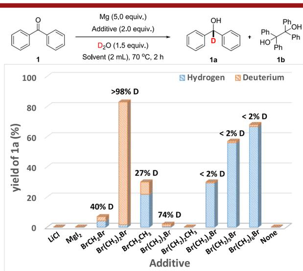
**Figure 2.** Reductive deuteration of ketones with different additives.
