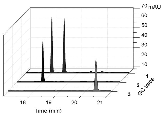
**Figure 2.** GC-trace 1: chemically prepared *all-rac*-**4a** (Chiral-DEX CB column) after derivatisation (see the Supporting Information). Peaks from left to right: (1*S*,3*S*)-**4a**, (1*R*,3*R*)-**4a**, (1*R*,3*S*)-**4a** and (1*S*,3*R*)-**4a**. GC-trace 2: enzymatically prepared (1*S*,3*S*)-**4a** (His-VF- $\omega$ TA). GC-trace 3: enzymatically prepared (1*S*,3*R*)-**4a** (ArRmut11- $\omega$ TA).
