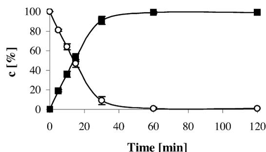
**Figure 1.** OCH (lyophilised crude extract, 20 mg mL<sup>-1</sup>) and CAL-B (Novozyme 435, 20 mg mL<sup>-1</sup>) catalysed conversion of diketone **1a** (50 mM) to (*S*)-**3a** (■) in DIPE:H<sub>2</sub>O:MeOH (97.5/2.5/1, v/v<sup>-1</sup>) at 30 °C, 120 rpm.
