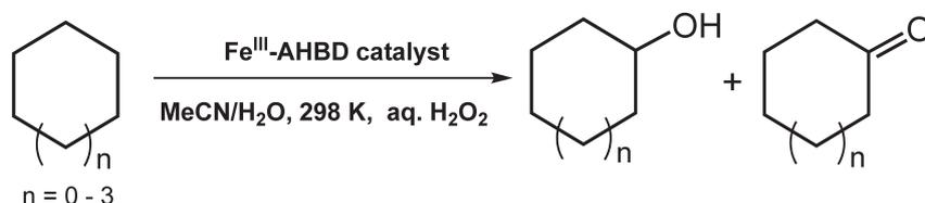
**Scheme 3.** Oxidation of cyclohexane using **3** or **4** as a catalyst precursor.
