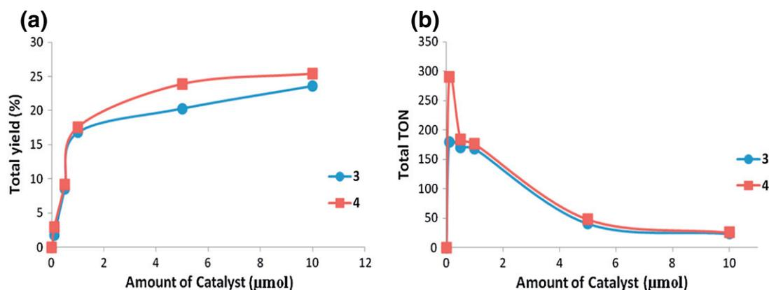
**Fig. 4.** Effects of the amounts of catalysts **3** and **4** on the total (cyclohexanone and cyclohexanol) yield (a) and TON (b), in the peroxidative oxidation of cyclohexane. Reaction conditions: CH<sub>3</sub>CN (4 mL), C<sub>6</sub>H<sub>12</sub> (1 mmol), H<sub>2</sub>O<sub>2</sub> (7.5 mmol), n(HNO<sub>3</sub>)/n(cat) = 10, 25 °C, 6 h.
