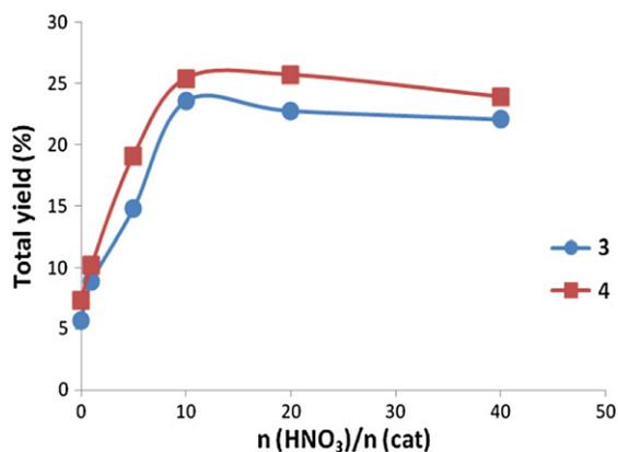
**Fig. 2.** Effect of nitric acid-to-catalyst molar ratio on the total (cyclohexanol and cyclohexanone) yield, in the peroxidative oxidation of cyclohexane. Reaction conditions:  $\text{CH}_3\text{CN}$  (4 mL),  $\text{C}_6\text{H}_{12}$  (1 mmol),  $\text{H}_2\text{O}_2$  (7.5 mmol), catalyst (10  $\mu\text{mol}$ ), nitric acid additive (0–400  $\mu\text{mol}$ ), 25 °C, 6 h.
