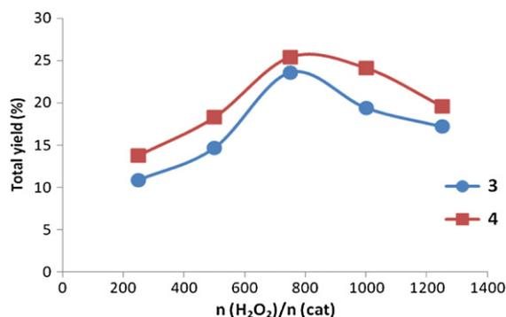
**Fig. 3.** Effect of the oxidant-to-catalyst molar ratio on the total (cyclohexanol and cyclohexanone) yield, in the peroxidative oxidation of cyclohexane. Reaction conditions:  $\text{CH}_3\text{CN}$  (4 mL),  $\text{C}_6\text{H}_{12}$  (1 mmol),  $\text{H}_2\text{O}_2$  (2.5–12.5 mmol), catalyst (10  $\mu\text{mol}$ ), acid additive (100  $\mu\text{mol}$ ), 25 °C, 6 h.
